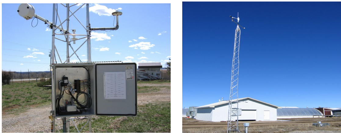
Figure 3 – Ute 1 Meteorological tower and weather resistant, surge protected enclosure box (left). The thirty-foot meteorological tower (right).
